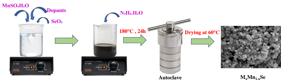
Figure 3.1 A schematic representation for the synthesis of M_xMn_{1-x}Se ( M = Co / Ni / Zn , x = 0.0, 0.01, 0.02, 0.03 )
