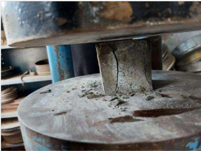
Fig. 3.17 Compressive strength test setup
