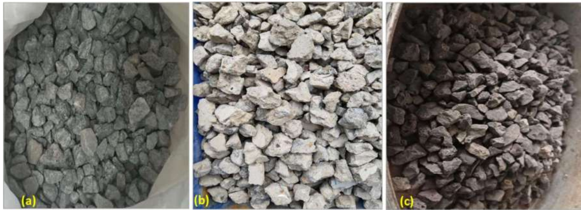
Fig. 3.1 Physical appearance of (a) natural granite aggregate (b) recycled concrete aggregate (c) ferrochrome slag aggregate
