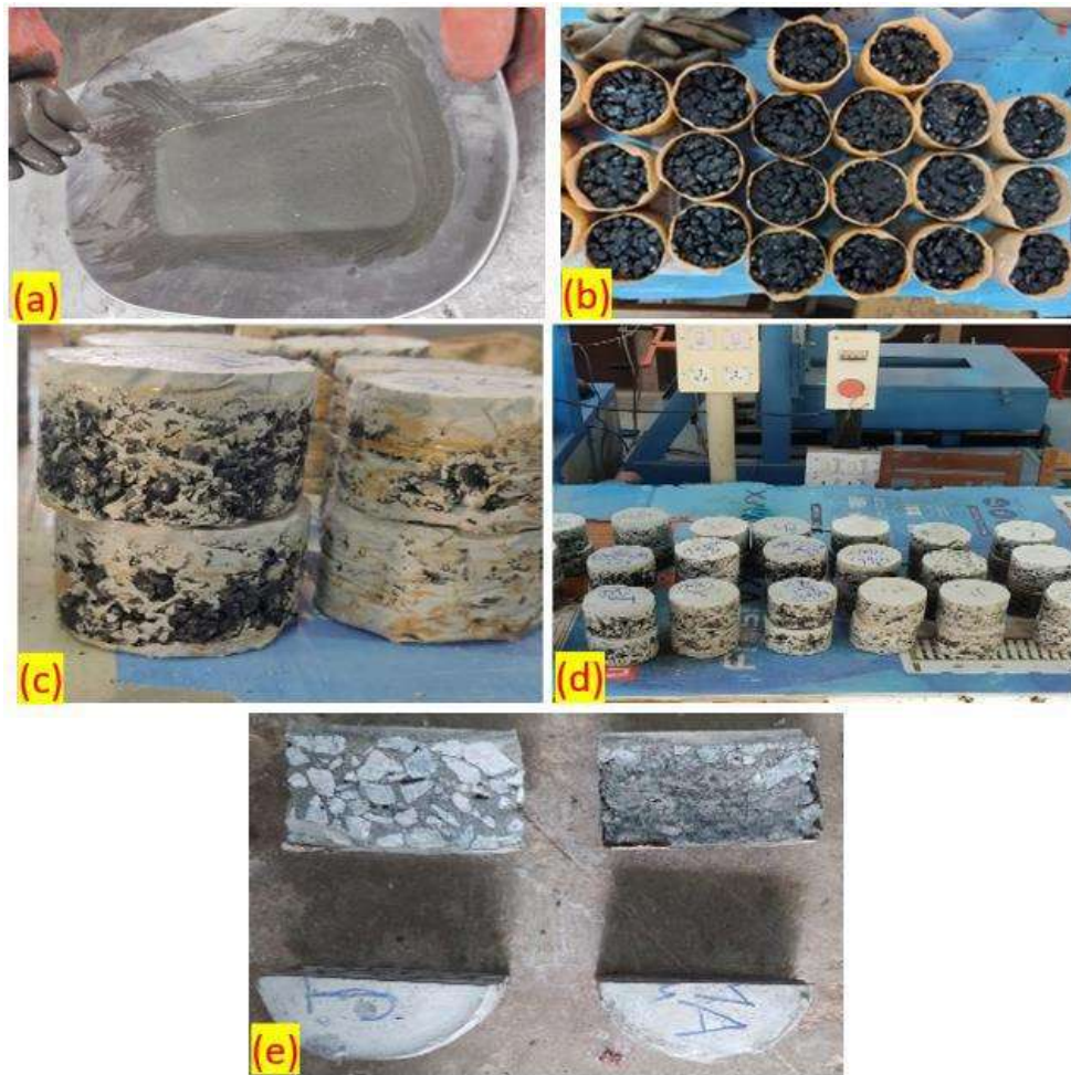
Fig. 5.3 (a) Grout (b) OGA specimens before grouting (c) SFA specimens: partially grouted specimens (on left) and full-depth grouted (on right) (d) Full-depth grouted SFA specimens (e) Visual inspection of full-depth grouting by cutting SFA specimens into halves
