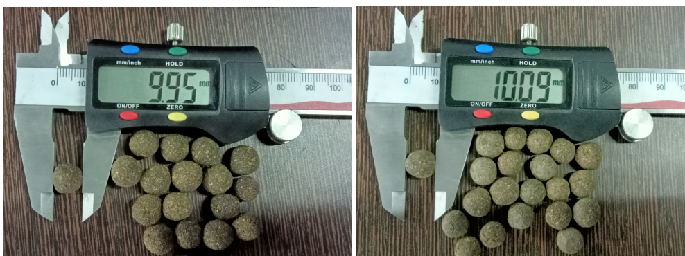
Figure 3.3: Actual size of metal-embedded natural composite desiccants
