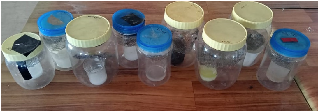
Figure 3.9: Photograph of moisture sorption isotherms rig
