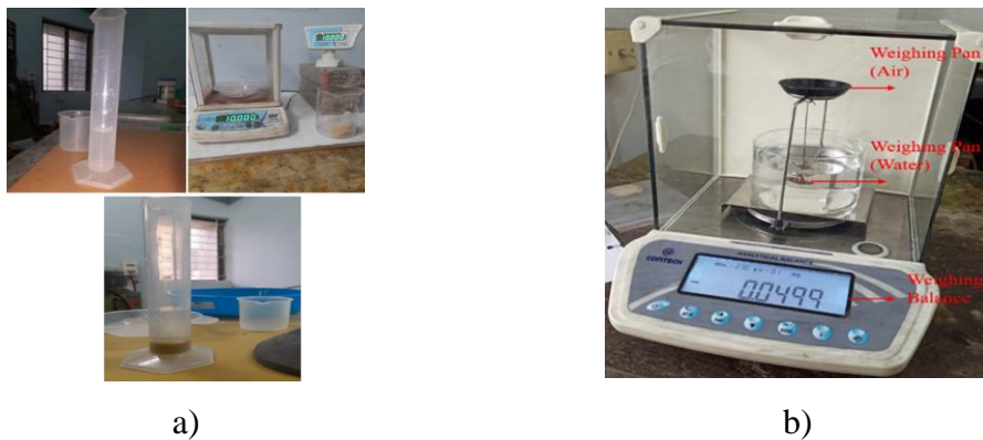
Figure 3.16 Density Calculation a) Conventional method, b) Density kit
