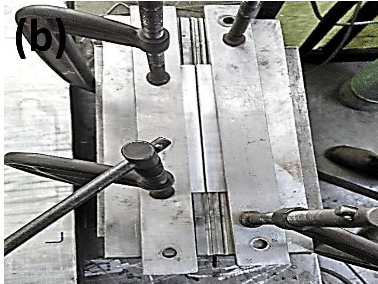
Fig. 3.2 Clamping set up to hold the specimens in a TIG and CMT (a) Side view (b) Top view.
