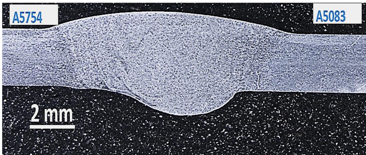
Fig. 4.96 Macrostructure of transverse section of the TIG welded A5754-H111 and A5083-H111 joint using ER5356
