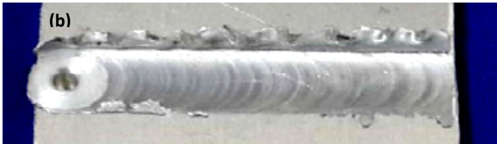
Fig. 2.9 (a) Schematic illustration of friction stir welding (FSW) process and (b) Friction stir welded surface (Dawood et al. 2015a)
