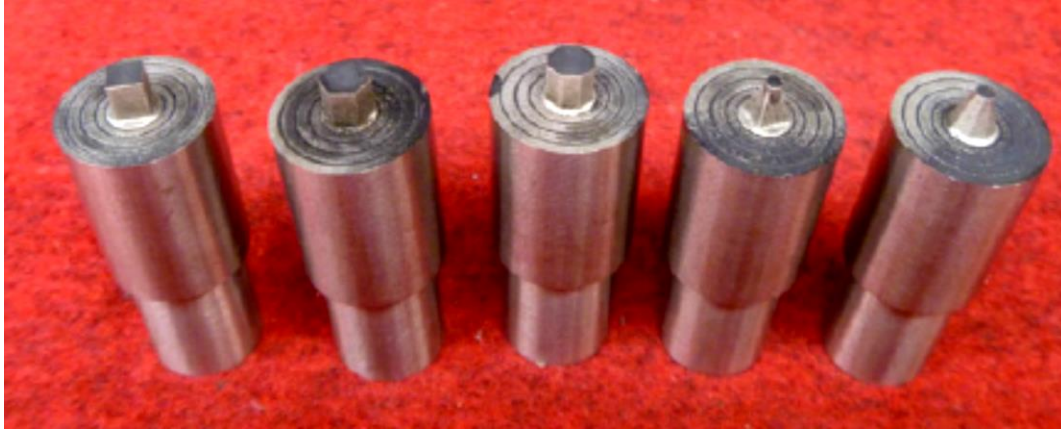
Fig.2.12 Different tool pin profiles of friction stir welding tool (Palanivel et al. 2012).
