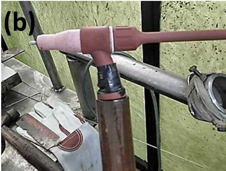
Fig. 3.4 (a) Tungsten inert gas (TIG) welding equipment and (b) Welding torch
