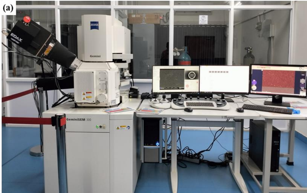
Figure 3.4 FESEM setup with EDAX and EBSD attachment.
