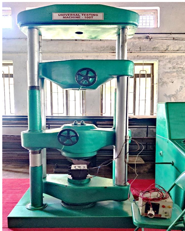
Figure 3.2 100-Ton UTM with MAF die and heating setup.
