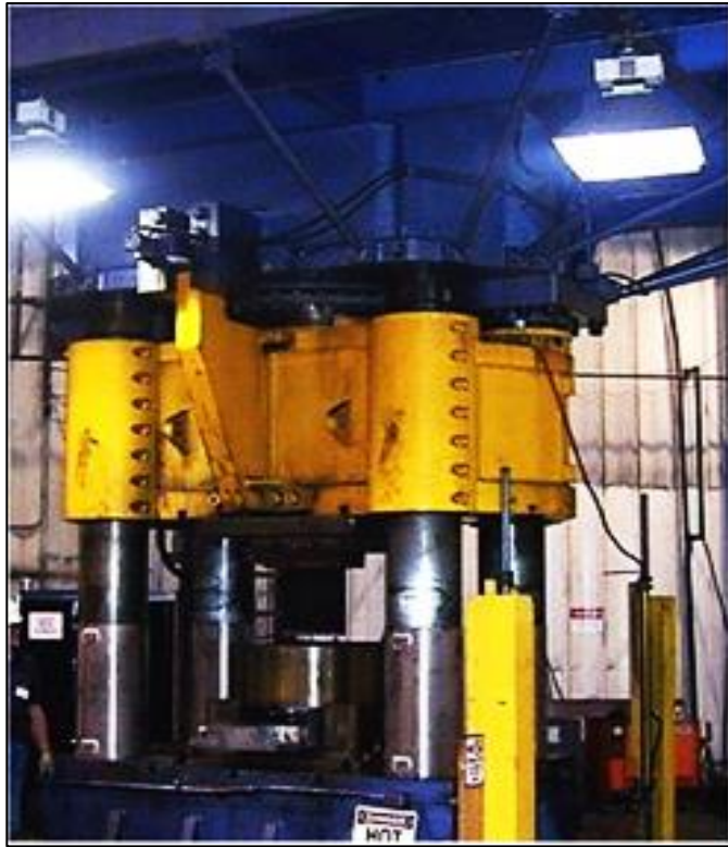
Figure 1.6 4000-ton hydraulic press with ECAP die assembly (Ferrasse et al. 2008).
