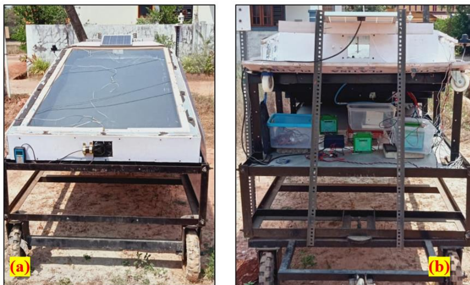
Figure 3.22 Details of the experimental setup of SAH (a) front side view (b) backside view.
