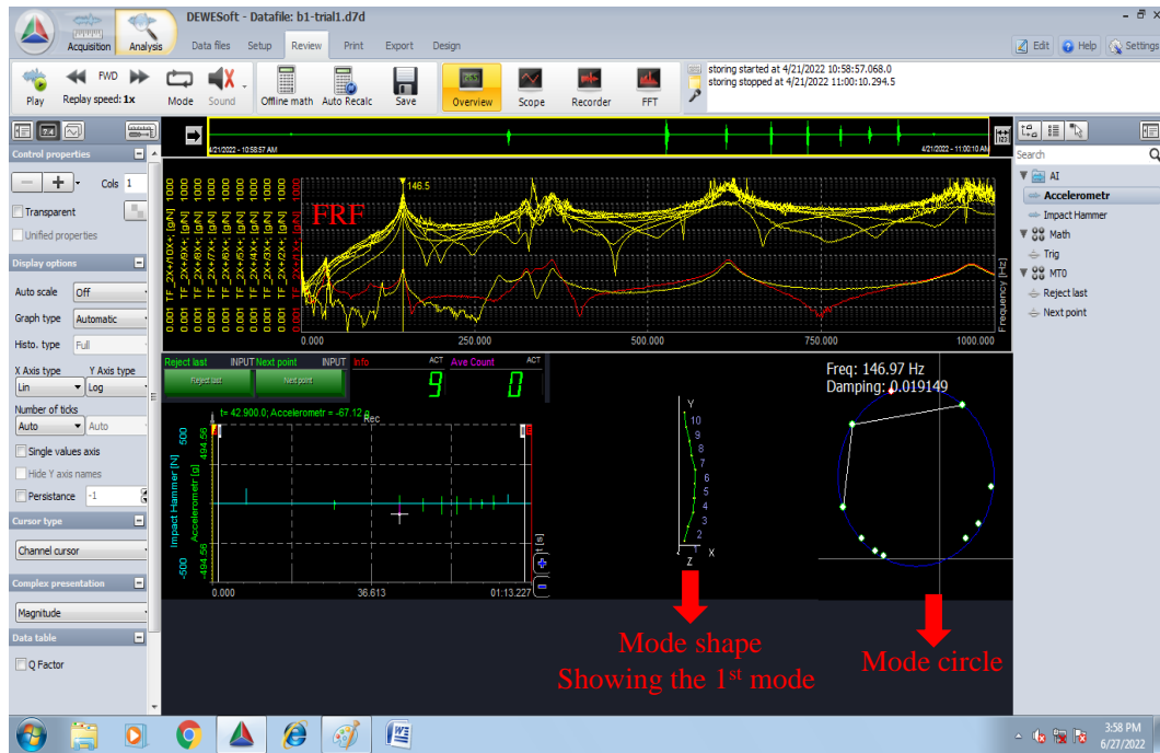
Figure 2.17. DEWESoft software showing FRF, mode shape and mode circle in the experimental modal analysis.
