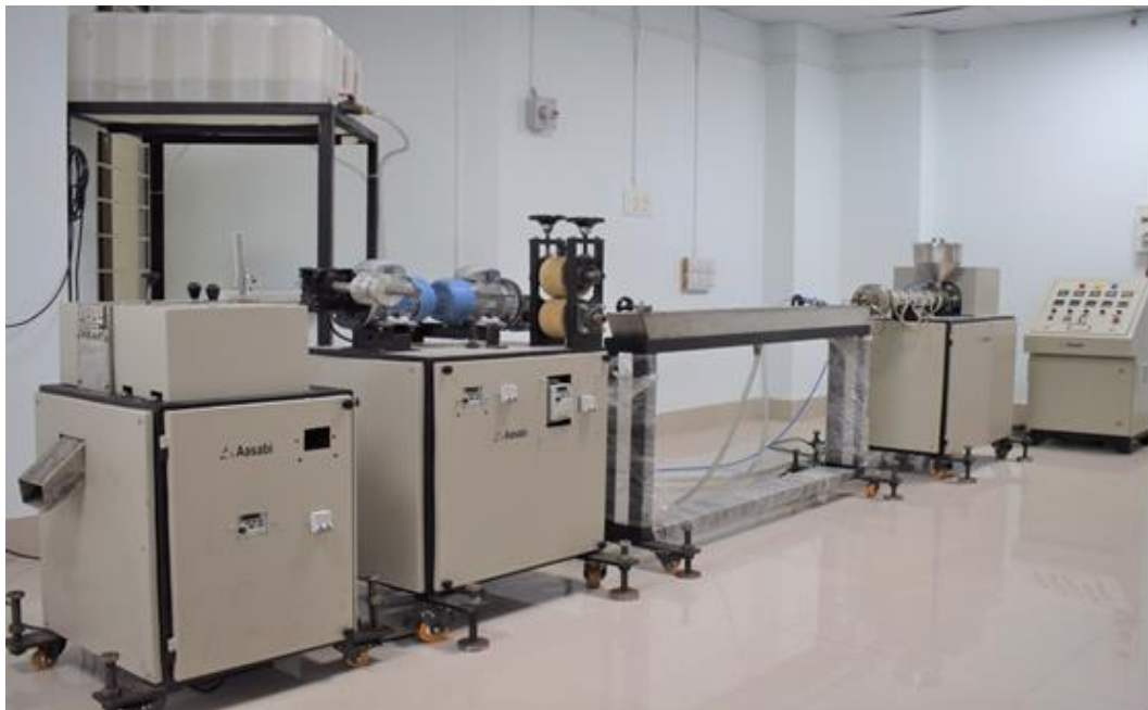
Figure 2.6. Experimental setup of the single screw extruder used in the current work.
