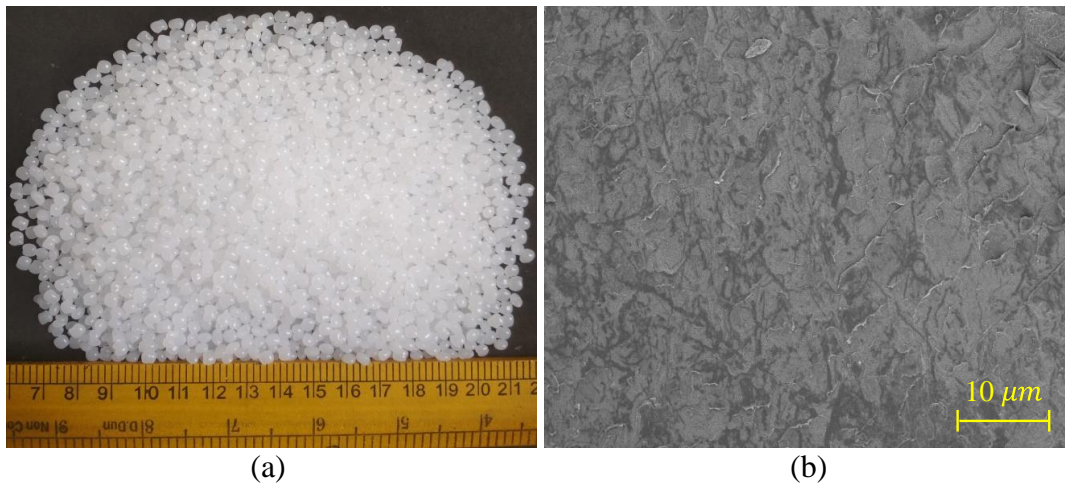
Figure 2.1. (a) Representative images of the as-received HDPE granules and its (b) SEM image.
