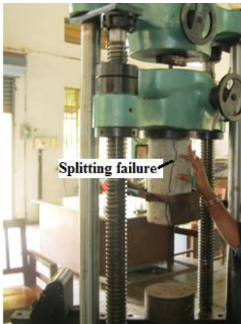
Fig.3.7: Occurrence of splitting failure
