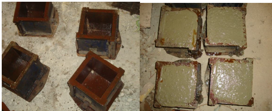
(a) Steel mould for auxiliary specimens
