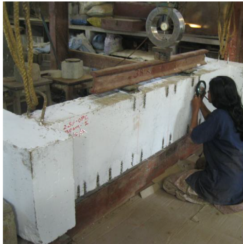
Fig.3.26: Observation of crack under magnifying glass
