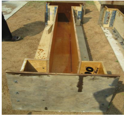
Fig.3.12: NBS beam specimen with Form work
