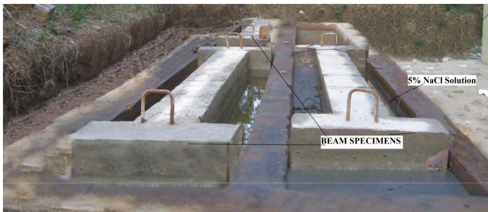
Fig.3.20: Accelerated corrosion of beam specimens
