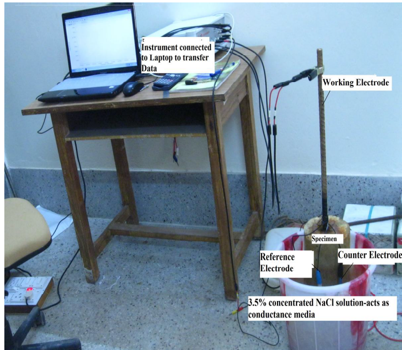
Fig.3.5: Corrosion monitoring test set up
