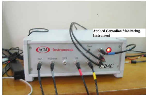
Fig.3.4: Corrosion monitoring instrument
