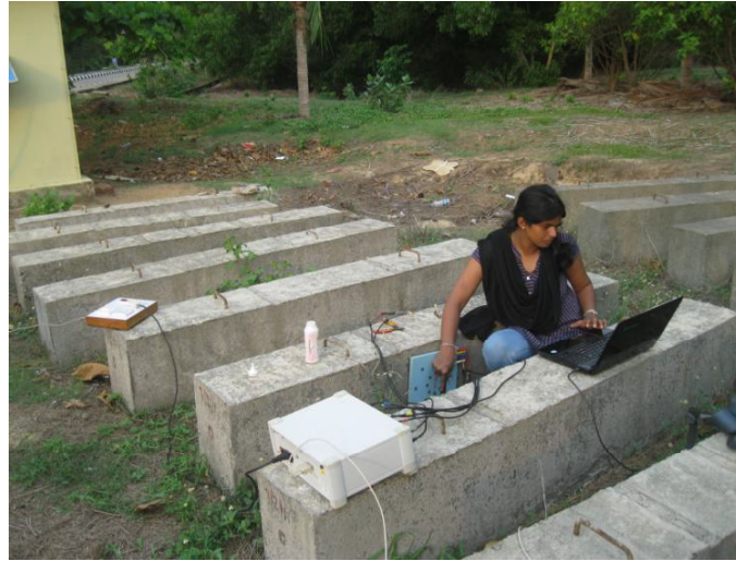
Fig.6.7: View of monitoring of naturally exposed beam near NITK beach
