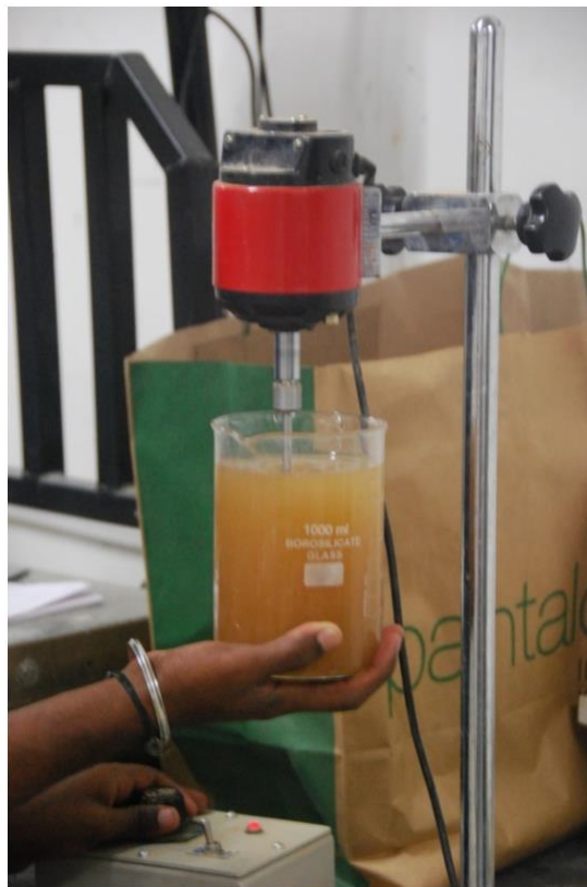
Figure 3.15 Mixing of clay particles for clogging test
