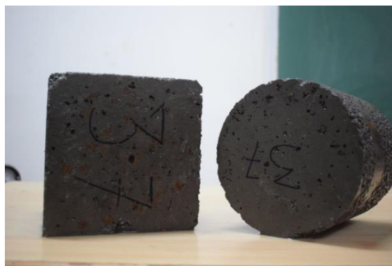
Figure 3.3 Cement paste drain at the bottom of concrete specimen
